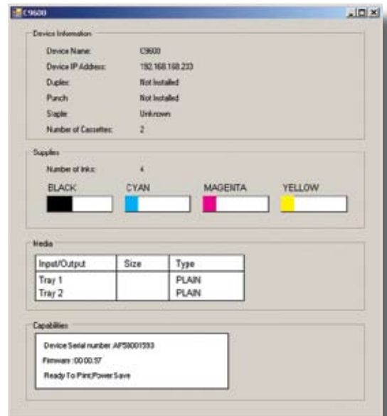
Bi-directional communication with printers to monitor status of the machine
