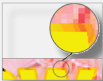
Miter trapping turned on - the brush shape tapers down at the corners to produce the best shape.
